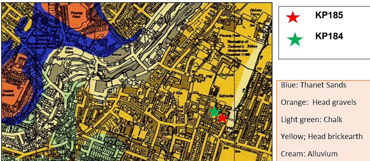
Figure 2b: Geological map of central Faversham, the same area as in Fig 2a 6 . Note the distinctive Davington Plateau (blue and orange) and Stonebridge Ponds (cream) areas.
