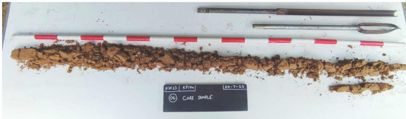
Fig 10: The core sample taken with the auger to a maximum depth of 3.2m.
